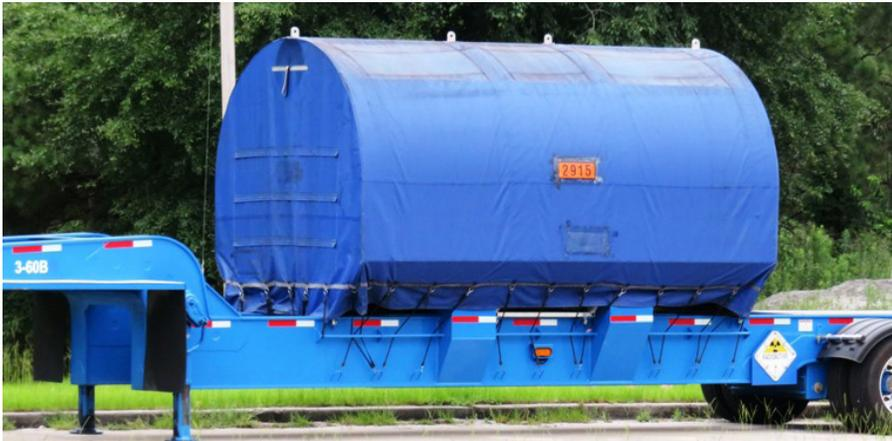
**Missing Markings!?!** At first glance, the communications for this conveyance may look good. How many orange panel markings are required on the outside of a personnel barrier (closed transport) when the orange panels on the bulk package contained inside, cannot be seen? The right answer is "4" orange panels, one on each side of the conveyance per 49 CFR 172.331(c). Also, how
