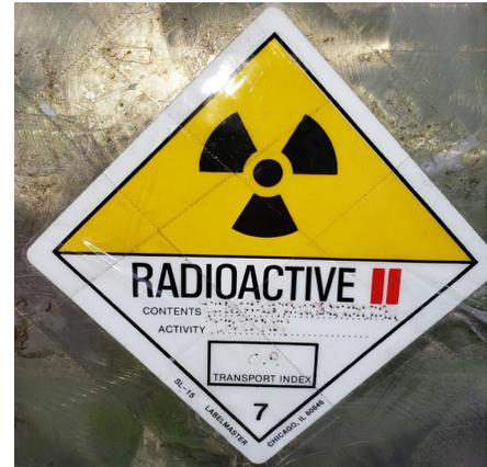
**Lacking Label?** What happened to the written information on this label? Looks like the ink got waterlogged or faded during transport. Be careful, all entries on DOT Radioactive specification labels must be legibly printed, manual or mechanical, and be durable weather resistant per 49 CFR 172.403(g). And a recommendation, if possible, fill out a few more extra labels for the driver to replace or cover over any bad package labels like this one.
