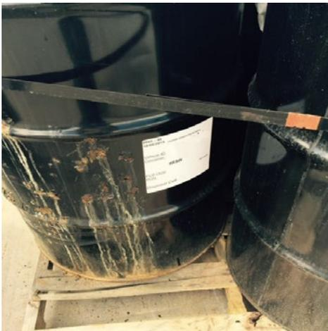
**Is it good to see the hazardous material in your drum shipment "eating" its way through the side? Should a shipper verify physical and chemical compatibility between anything inside the package and package's construction material?**
